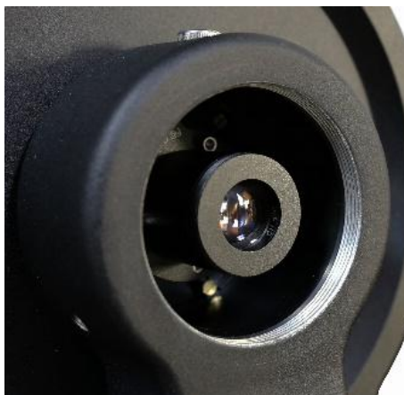
Figure 20. CEM120 with an installed iPolar electronic polar scope
